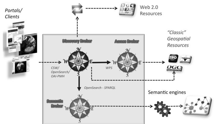
Fig. 3. The EuroGEOSS brokering framework includes different multidisciplinary EuroGEOSS Brokering components: The Discovery broker, the Access broker, the Semantic broker (Discovery Augmentation Component) and the adaptors to Web 2.0 resources.
