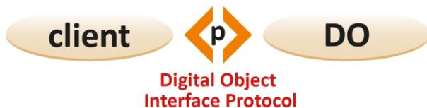
Figure 10 describes a typical client-server interaction with actors on both sides which have knowledge about what a DO is. At the right side it could be typically a repository with some services which can transform DOIP based interactions to the specific solution of data organization and modeling.
