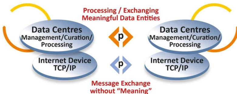
Figure 1 indicates the two layers of exchange in the Internet. At the bottom level is the datagram exchange between Internet Devices based on TCP/IP. At the top level is the exchange of meaningful information which needs to be supported by a dedicated protocol.
