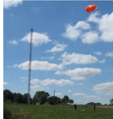
Balloon-borne turbulence probe (CNRM, 2010)
