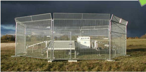
UHF radar wind profiler (150-3000 m height cover)
