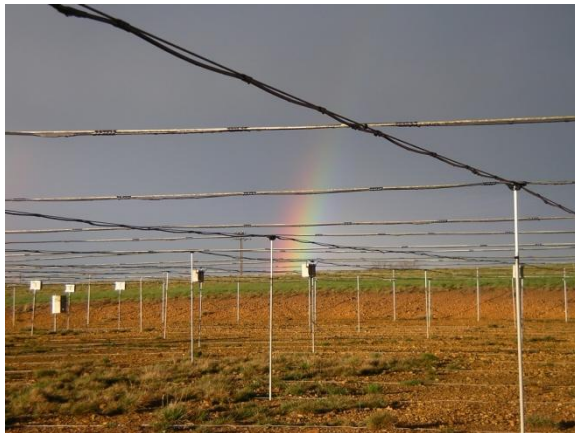
VHF radar wind profiler (1.5-16 km height cover)
